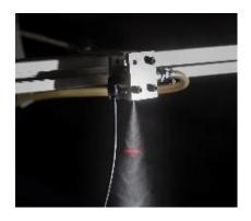
As two properly configured laser beams intersect, the light beams set up an interference pattern. As a droplet passes through this interference pattern, it scatters the light from the pattern in a burst of reflected light. The properties of the scattered light depend on the droplet size. The bursts of scattered light are captured by a receiver, and are converted to an electrical signal, which is interpreted by software to calculate the droplet size.
