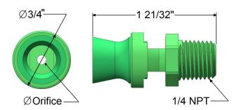
This capacity chart provides the flow of water through the nozzle orifice at various pressures and the expected circulation rate.
